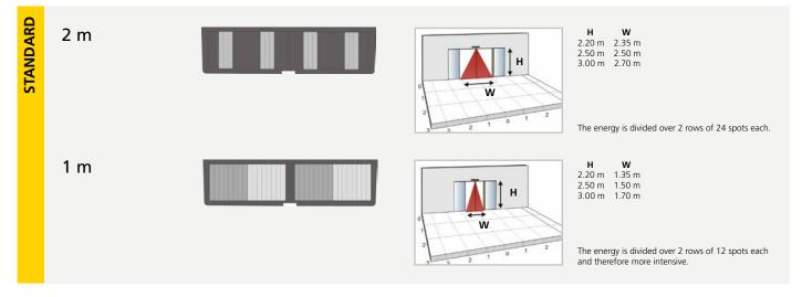
Furthermore, there are specially designed, so called masked prisms to adapt the detection field to your specific needs (sold individually). **Caution**: Do not mask the prisms yourself. This could lead to unsafe door installations.
