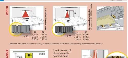
**TIP:** Launch an **ASSISTED SETUP** to verify wiring, position of the curtains and correct functioning of the sensor. It is recommended to clean the optical parts at least once a year or more often if required due to environmental conditions.
