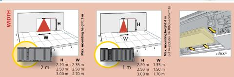
Detection field width indicated according to conditions defined in DIN 18650 and including dimension of test body CA.
