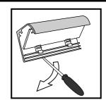
• Use a screwdriver to remove the plastic supports from the modules
