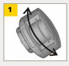
Adjust the lateral position of the detection field.
