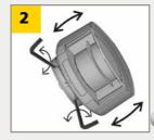
Adjust the tilt angle of the detection field with the hex key.
