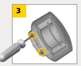
Lock the position of the mounting bracket to avoid malfunctioning in case of extreme vibrations.
