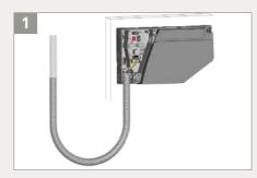
Take the flexible tube and determine how long it should be in order to reach the door controller.
