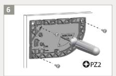
Fasten the 3 screws using a Pozidrive screwdriver.
