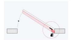
Optimised protection of the pinch zone on hinge side and opposite hinge side
