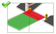
Make sure to place the detection field parallel to the boom.
