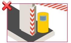
Do not cover the front face of the sensor with glass or plastic.
