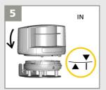
Position the housing on the mounting base.
