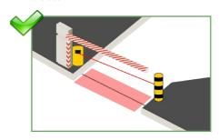
When using the safety, place the sensor just behind the barrier. This way the safety field protects the area around the boom.
