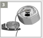
Open the protection cover, plug the connector and position the cable in the slit.
