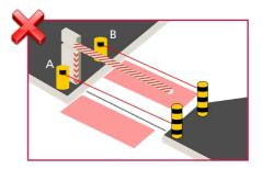
When using the safety, do not place the sensor before the barrier (A) or more than 40 cm after the boom (B). The area around the boom is not safe.
