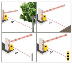
The sensor has to learn a reference when the safety field is the only protection against contact between the vehicle and the boom.
