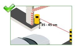
Install the sensor at a mounting height of 35 - 45 cm. If the barrier is only used by trucks, the mounting height can be increased.
