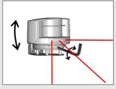
Adjust the tilt angle of the detection field witht the hex key if necessary.
