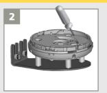
Position the mounting bracket and fasten the 4 screws firmly in order to avoid vibrations.
