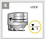
Turn the sensor until the two triangles are face to face.
