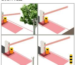
If the safety field is the only protection against contact with the boom, the safety field of the sensor must be situated right under the boom.
