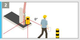
Use a white paper to verify the position of the 0° laser beam. The reference point can be adjusted on any object at the end of the boom or farther away. Its surface should be +/- 10 cm and it must be firmly fixed.
