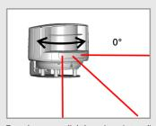
Turn the sensor slightly on its axis to adjust the lateral angle of the sensor to place the 0° laser spot on the reference.
