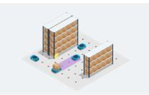
Deliver precise distance measurement data to the AGV's controller at a high frequency, allowing it to accurately **identify obstacles** within its trajectory and **react flexibly** by adapting its path.
