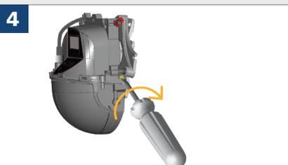
Carefully lock the sensor position by firmly fastening the angle lock screw. Make sure the red spots have not moved.
