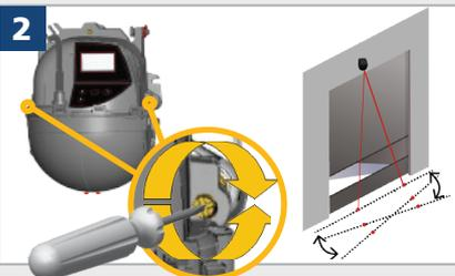
Make sure the curtain is **parallel** to the door by adjusting one or both screws on the side.
