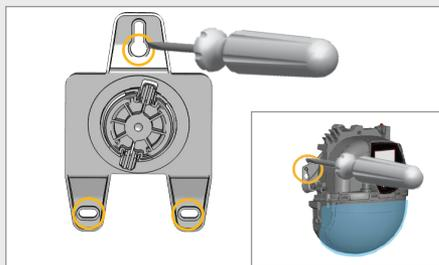
Screw the mounting bracket on the wall. You can also install the sensor directly without using the mounting bracket.
