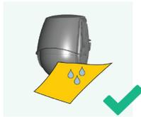
Wipe the laser window with a soft, clean and damp microfibre cloth. We recommend using optical lens cleaner.
