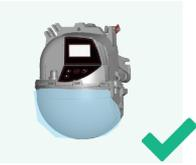
Keep the protection film during the mounting of the sensor. Remove it before launching a teach-in.
