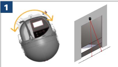
Rotate the sensor in order to align the centre of the red spots with the centre of the door.
