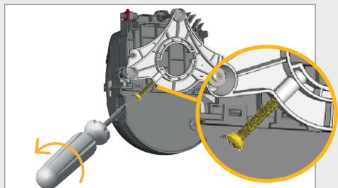
Unscrew the angle lock screw if necessary.
