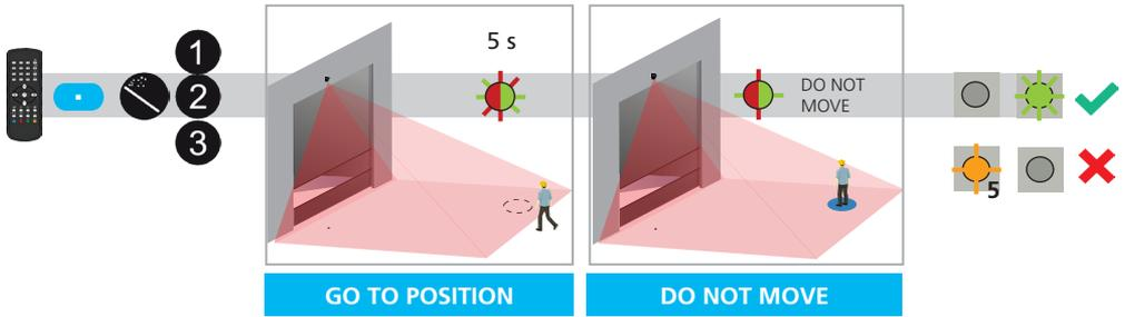
Launch a pull cord teach-in by remote control. You can create 3 different pull cords in the scanned area.
