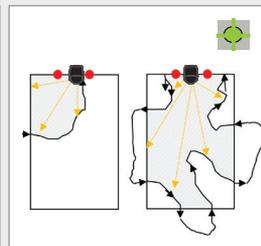
Some examples of walk teach-in. TIPS : Start the walk teach-in when the LED is flashing green. Walk slowly. Never start or walk too close from door center. Finish tracing outside the scanning area.
