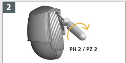
Lock the cover by turning the lock screw clockwise.
