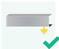
The metal base on which the sensor is mounted, must be correctly earthed.
