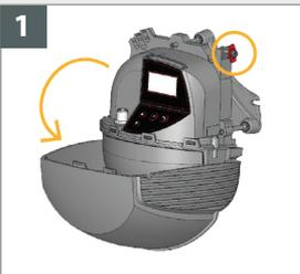
Before opening the sensor, make sure the cover is **not locked** (red cover lock).
