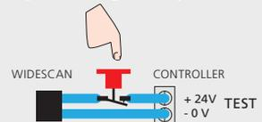
TIP: Add a push button in serie with the test line (24VDC). Pushing this button during 3 sec (cuts supply of input) launches a background teaching.
