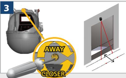
Position the curtain **closer to or further away** from the door by turning the screw at the top.
