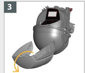
If needed, remove the cover completely before installing the sensor.
