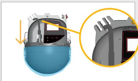
Plug the connector and pass the cable through the cable passage without making a loop.
