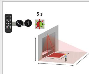
Launch with remote control or LCD. The teach-in starts after 5 seconds once performed on the remote control ( 60s if LCD). Ideally and when possible, start outside the scanning area.
