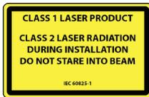
The device emits invisible (IR) and visible laser radiations. The visible laser beams can be activated during the installation process to adjust precisely the position of the detection field.
