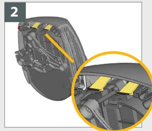
To open the top cover, pull both flags while tilting the cover away from its initial position.
