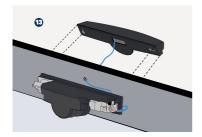
13. Install the second module following the same steps and connect it to the BLUESPIN cable.
