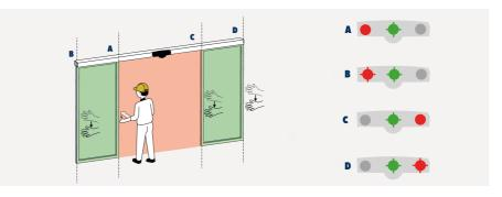
7. Once the door is completely closed and all the LEDs are OFF, the teach-in is completed. Check the correct positioning of the safety fields by placing an object in the detection field. If needed, adapt them manually.
