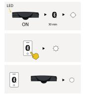
At power ON or after a power cycle, the Bluetooth® is activated for 30 min and the Bluetooth® LED is flashing white.
