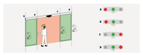
Once the door is completely closed and all the LEDs are OFF, the teach-in is completed. Check the correct positioning of the safety fields by placing an object in the detection field. If needed, adapt them manually.
