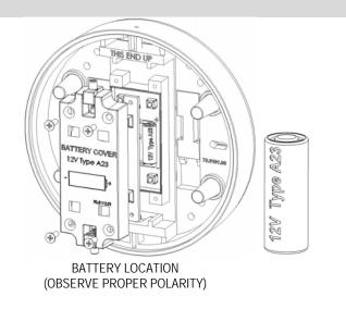
To replace the battery, remove the faceplate and the 4 screws holding the battery cover to expose the transmitter assembly. Replace the battery with a fresh 12V, type A23 battery and reassemble the push plate.
