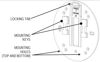
To install the mounting plate, screw a minimum of two countersunk head screws (#8) into a solid surface through the holes in the mounting plate. The mounting plate must be mounted so that the text side is facing up.
