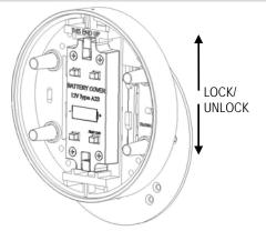
To attach the housing to the mounting plate, place the housing over the mounting keys on the mounting plate, and then slide the housing downward until the locking tab engages the housing. To remove the housing, press in the locking tab and reverse this procedure. To securely lock the plate, put an additional screw through both the housing and the mounting plate.
