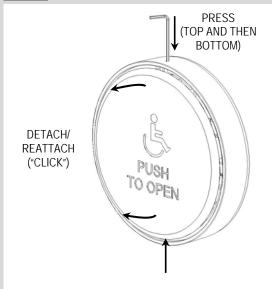
To assemble or disassemble the push plate, use the enclosed hex key (or similar diameter tool) to press in and release the spring clips from the faceplate bracket. The spring clip will need to be engaged / disengaged from top and bottom, one at a time. When the spring clips are correctly engaged, they will make a "click". It may be necessary to rotate the faceplate slightly to have them lock correctly.
