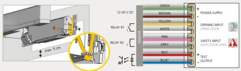
The door control unit and the door cover profile must be correctly earthed.
