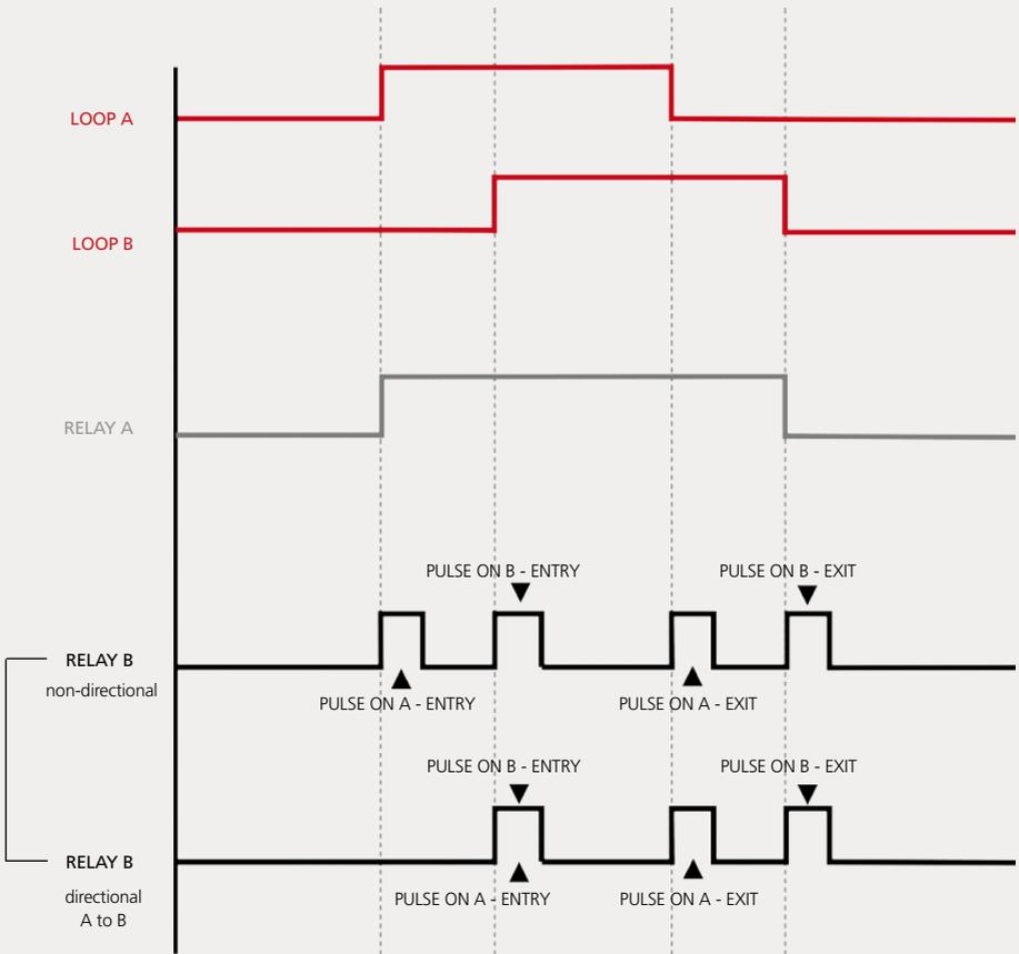
In order to enable directional detection, the 2 loops should be installed close to each other. When a vehicle is not detected anymore on loop A whilst entering loop B, no relay output will be triggered.
