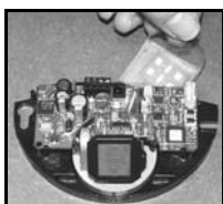
Remove the narrow sensing field antenna from its location.
