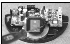
Carefully remove the clamp of the antenna and the wide sensing field antenna.
