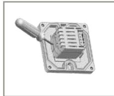
If you need to unclip the radar module from the front face, use a screwdriver or a pencil.
