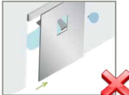
Do not place the sensor in the opening range of the door.
