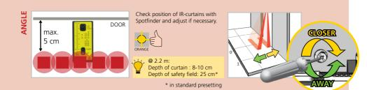
The size of the detection field varies according to the mounting height of the sensor.
